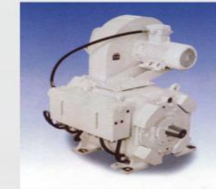
YJ14 And YJ14A Variable Frequency Speed Regulating Asynchronous Motor Used as Mud pump, Rotary Table and Drawworks motor Rated Horse Power: 550 HP, 550 V, 582 A, 660RPM, 33.4 HZ
