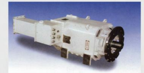
YZ10 DC Motor Used as mud pump, Rotary Table, and Drawworks motor Rated Horse Power: 1100 HP, 750 V, 1150 A, 1060 RPM
