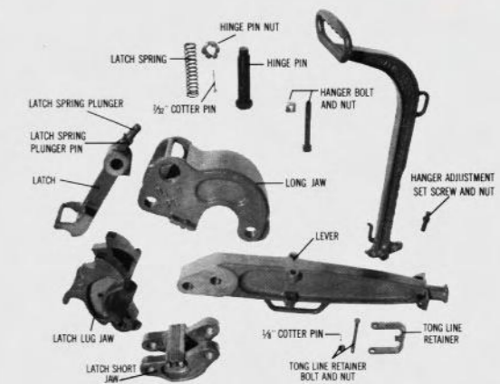
Parts View, BJ Types F and LF Tongs.
