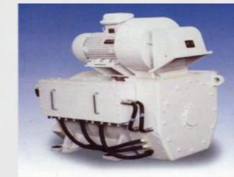
YJ21 Variable Frequency Speed Regulating Asynchronous Motor Used Mud pump, Rotary Table and Drawworks motor Rated Horse Power: 1100 HP, 660 V, 850 A, 800 RPM, 40.5 HZ
