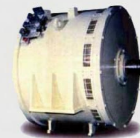
YZ08 And YZ08A DC Motor Used as mud pump, Rotary Table, and Drawworks motor Rated Horse Power: 1100 HP, 750 V, 1150 A, 970 RPM,
