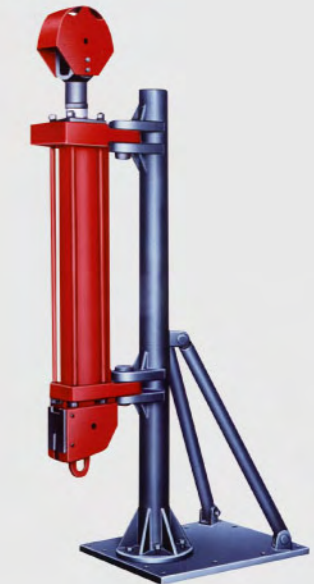
KELLY SPINNER (KS) (HT17) is designed and manufactured under Varco 6600 (Pneumatic Kelly Spinner) and 6800 (Hydraulic Kelly Spinner) designs, which is used for rotating drill pipe slowly, for limited rathole and mousehole drilling, and for making fast Kelly connections. This unit is completely reversible, the driller can spin out, as well as spin in, and when making connections, therefore, spinning chains are not required any more.
