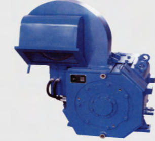
YZ08F DC Motor Used as mud pump, Rotary Table, and Drawworks motor Rated Horse Power: 1100 HP, 750 V, 1150 A, 1060 RPM
