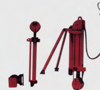
KELLY SPINNER (KS) (HT17) is designed and manufactured under Varco 6600 (Pneumatic Kelly Spinner) and 6800 (Hydraulic Kelly Spinner) designs, which is used for rotating drill pipe slowly, for limited rathole and mousehole drilling, and for making fast Kelly connections. This unit is completely reversible, the driller can spin out, as well as spin in, and when making connections, therefore, spinning chains are not required any more.
