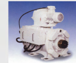
YJ23 Variable Frequency Speed Regulating Asynchronous Motor Used as Mud pump, Rotary Table and Drawworks motor Rated Horse Power: 825 HP, 600 V, 714 A, 660 RPM. 33.5 HZ
