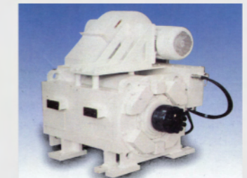
YJ27 Asynchronous Traction Motor Used as Drawworks motor Rated Horse Power: 320 HP, 380 V, 444 A, 686 RPM.
