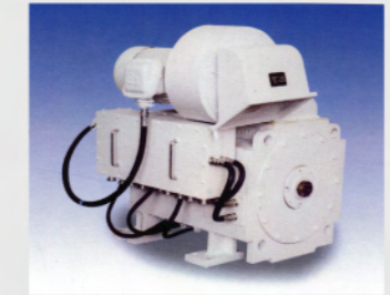
YJ19, YJ19A AND YJ19B Variable Frequency Speed Regulating Asynchronous Motor Used Mud pump, Rotary Table and Drawworks motor Rated Horse Power: 550 HP, 600 V, 517A, 660 RPM, 33.5HZ
